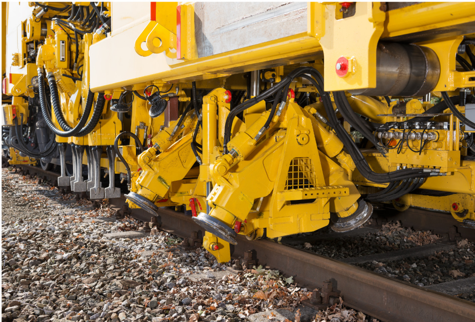
(a) Roll lifting clamps and double-flange lining rollers of a plane tamping machine
