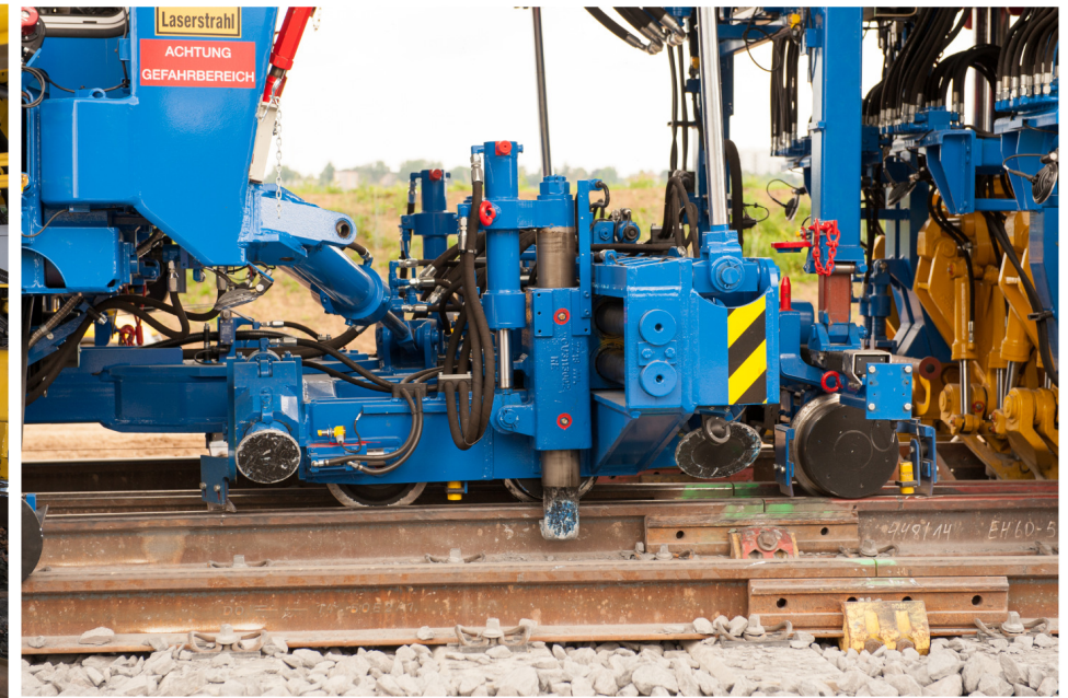
(b) Roller lifting clamps with lifting hooks and lining rollers for universal use in turnouts
